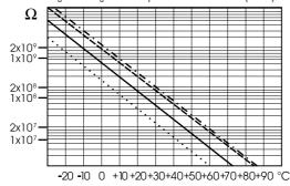
Since the resistance of the pH electrode is in the range of 50 - 200 Mohm, the current across the membrane is in the pico Ampere range. Large currents can disturb the calibration of the electrode for many hours.
